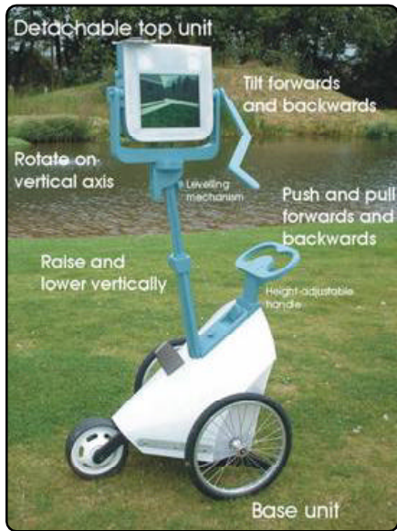
Figure 3-11. On the other end of the spectrum from the IBM Everywhere Display or the Social Floor is the Augurscope. The Augurscope provides a physical interface between the environment and a virtual model of the land as it existed in medieval times when Nottingham Castle stood on the same site.
