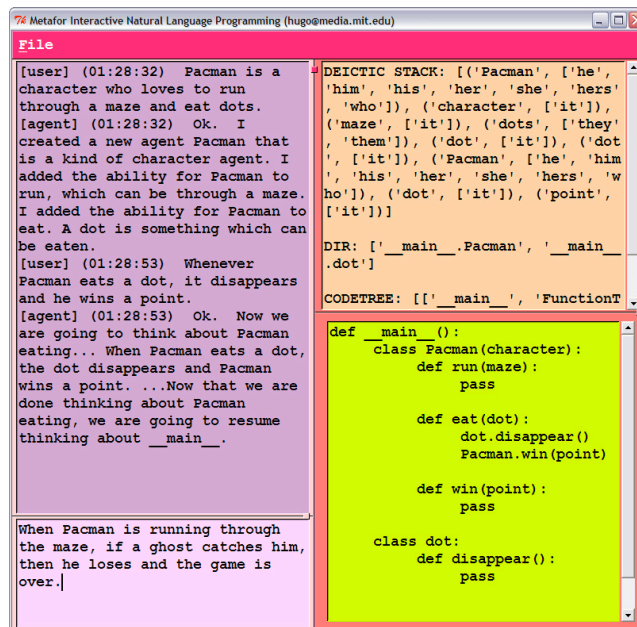
Fig. 1. The Metafor natural language programming system. At the lower left is the user's natural language input. At the lower right the automatically generated code. The two top windows trace the parser's actions and are not intended for the end user.
