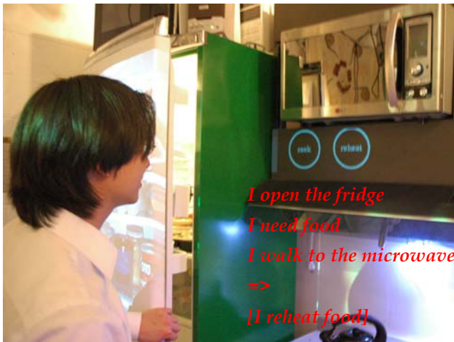
Figure 2. When a user opens the fridge and stands in front of the microwave, the kitchen recommends an enhanced microwave interface for him to ‘cook’ or ‘reheat’ food.
