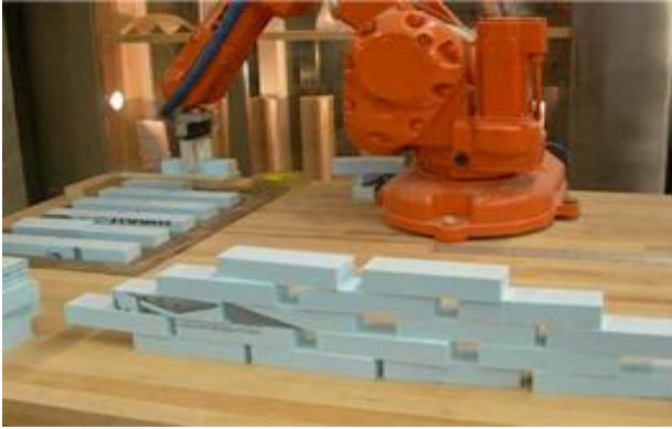
Figure 6. Vertical wall configuration as performed by the digital fabrication device.
