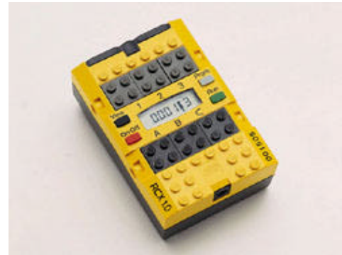
Figure 5 the LEGO™ RCX Brick used in PCTA
