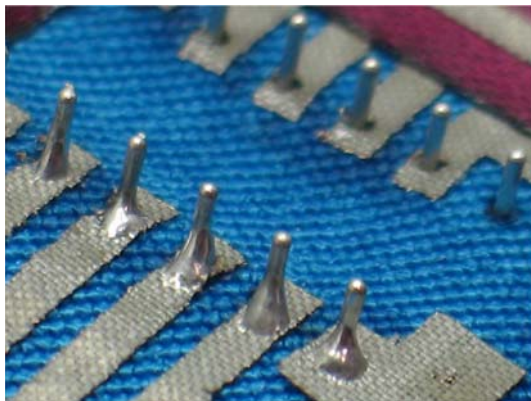
Fig. 2 Solder joints on a fabric PCB
