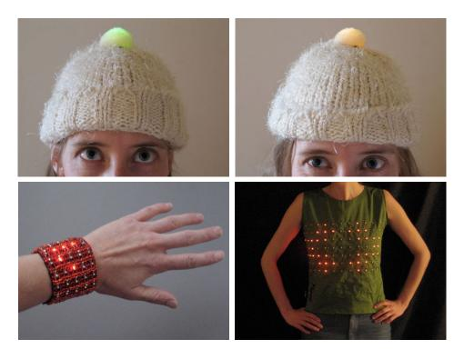
Figure 6. Top: A temperature-sensing hat. Bottom: Wearable LED displays.
