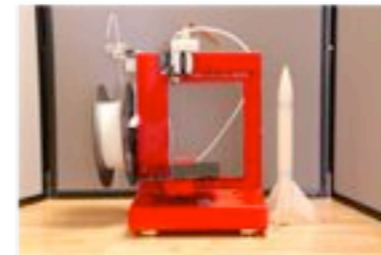
3D printing: small FDM machines using ABS and PLA
