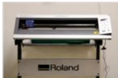
Vinyl cutter used for graphics, flexible electronics, antennas and sensor structures
