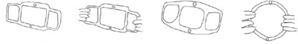
Figure 3: A VideoCube with handles was transformed into the Tangicam picture-taking frame, removing the controller and leaving only the handles.
