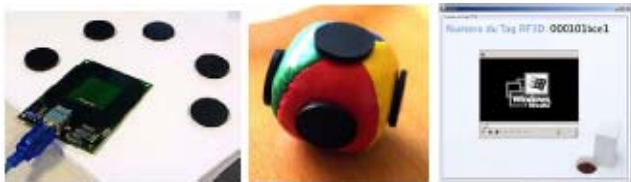
Figure 2: (left) Video cube components: RFID tags and wireless controller (center) Videocube input device (right) Screen display controlled by Videocube
