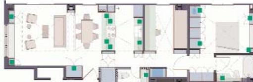
Environmental Sensors: Temp., Humid., etc.
