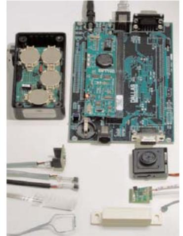
"Tini" micro-controller and some of the sensors embedded in cabinetry.
