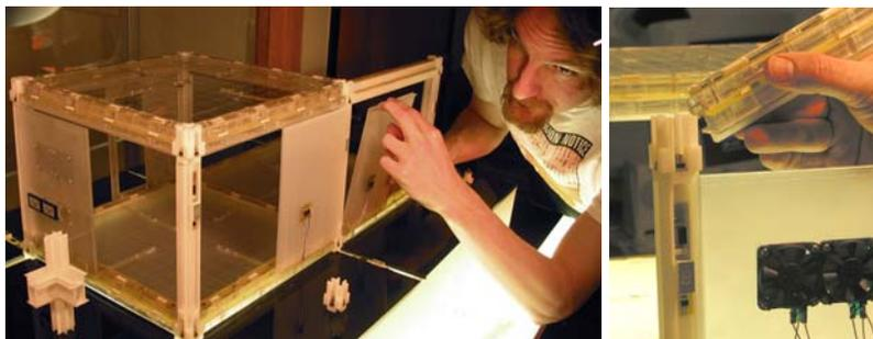
Figure 2. House\_n pultrusion chassis and communication: 1/12th scale model of a post and beam chassis to study embedded computational technology that allows newly-introduced devices to announce their presence on the network (McLeish, 2003).
