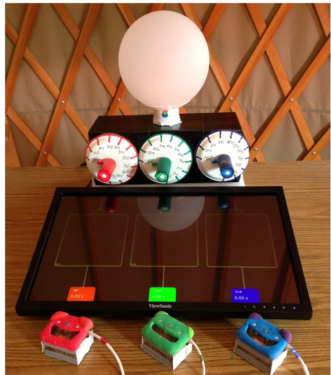
Figure 3. EnergyBugs system with energy harvesting Bugs, display, and the Lamp.
