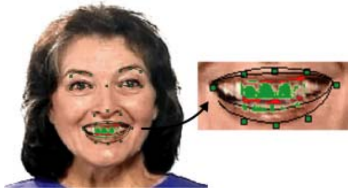
Figure 1.4. The facial affect analyser extracts facial feature points on the face, and uses that along with colour information to determine facial actions. A close up of the mouth feature points, the inner and outer lip contours, and additional colour information (teeth, aperture) is shown on the right. The pose estimation points (e.g. nose tip and nose root) are tracked to recognise head gestures (Video courtesy of the Autism Research Centre, Cambridge).
