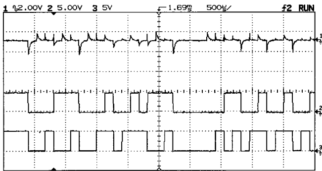
Fig. 5. Top trace: received signal induced by four coded waveforms. Middle and bottom traces: two of the four transmit channels.
