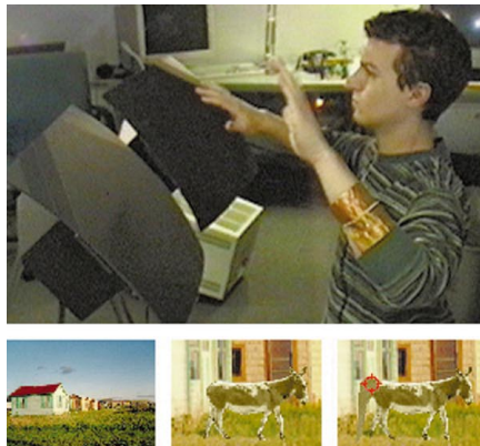
6 A user interacting with the FishPad using the one-handed configuration to browse through a watch catalog (right) and a two-handed implementation to play a virtual “pin-the-tail on the donkey” (left).
