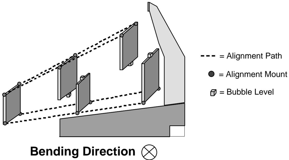
**Figure 7: Alignment Paths in the Muon Endcaps**
