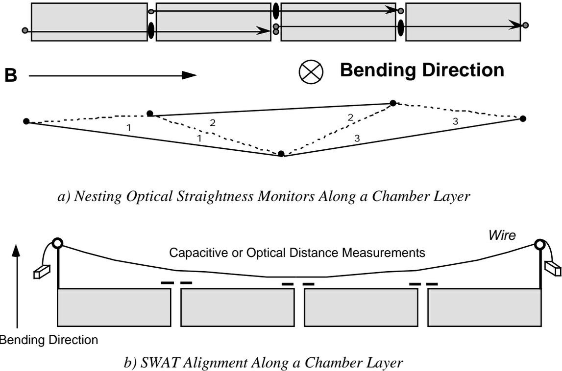
**Figure 5: Multipoint Alignment along Beam Axis**
