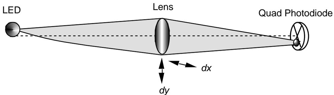
Figure 1: The Basic Straightness Monitor
