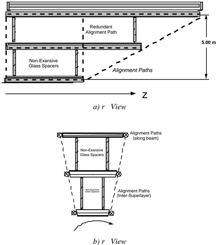
**Figure 4: Straightness Monitor Paths in Muon Chamber Barrel**
