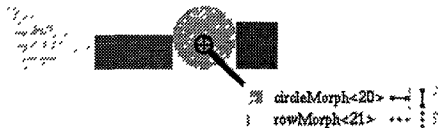
Figure 8. The core sampler with proxies for the two submorphs at its cross hairs, a circle and the row that contains it. The small square on the left side of each proxy shows the color of the associated morph. When the mouse is pressed over this square, a bright-colored frame is temporarily drawn around the submorph to help the user locate the submorph visually. As an accelerator for experienced users, holding the shift key while pressing the mouse over the square extracts the given submorph, while holding the shift key as a morph is dropping onto the square embeds the dropped morph in the given morph.
