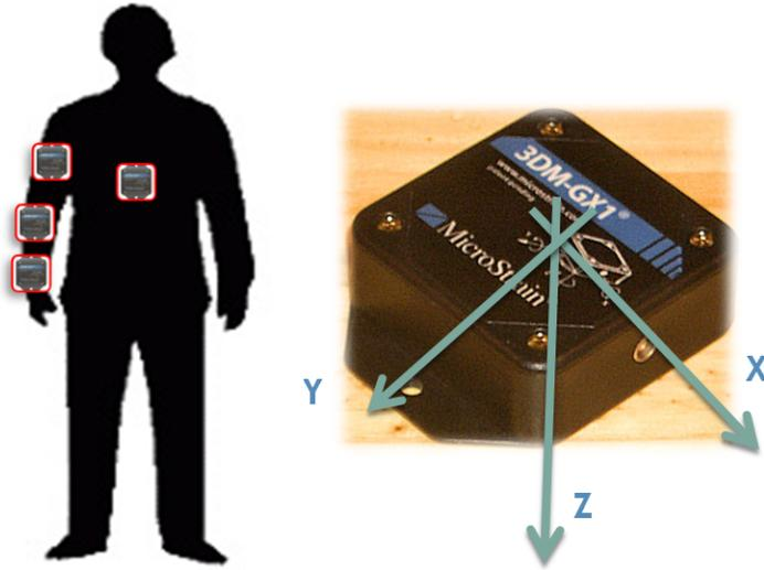
Figure 1: Left, IMU placement. Right, the 3DM-GX1<sup>®</sup>.
