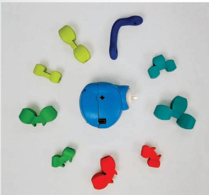
► Topobo: Kinetic 3-D constructive assembly system.
