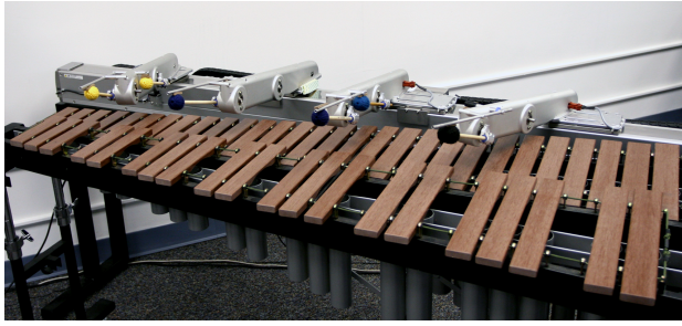
Fig. 1. Overall view and detail view of the robotic marimba player Shimon
