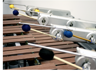
Fig. 1. Overall view and detail view of the robotic marimba player Shimon
