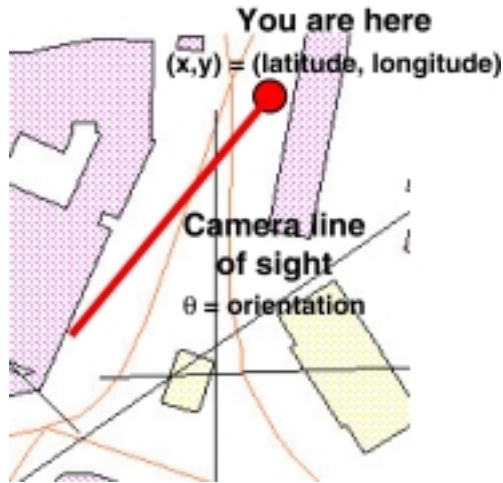
Fig. 3. A segment of the ArcView GIS map for Cambridge, Massachusetts. The red dot shows the current camera position at a GPS coordinate. Orientation is used to trace a vector from the camera origin along its line of sight. The current algorithm simply returns the first building that intersects the line of sight vector
