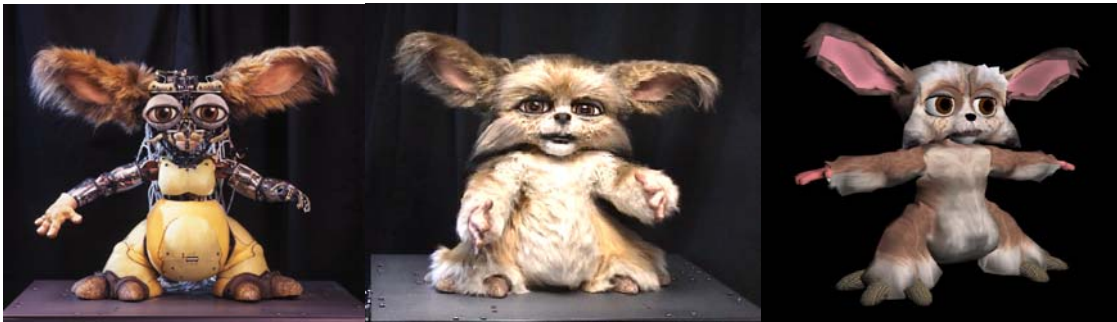
Figure 1: Leonardo is a 65 degree of freedom (DoF) fully embodied humanoid robot that stands approximately 2.5 feet tall. It is designed in collaboration with Stan Winston Studio to be able to express and gesture to people as well as to physically manipulate objects. The robot is equipped with two 6 DoF arms, two 3 DoF hands with tactile sensation, an expressive ( 24 DoF) face capable of near human-level expression, an active binocular vision system (4 DoF), two actively steerable 3 DoF ears, a 4 DoF neck, with the remainder of the DoFs in the shoulders, waist, and hips. A speech recognition and understanding system (developed by and used in collaboration with the Naval Research Lab) allows the robot to engage in task-oriented dialogs with a human. The left picture shows the robotic structure, the center picture shows the robot when cosmetically finished, the right shows a simulated version of the robot.
