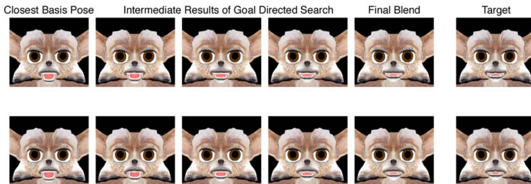
Figure 9: Goal-Directed Search Towards Target Pose. Once Leonardo has mapped the human's pose onto its own joint space, creating a target pose, the robot executes a goal-directed search of its possible facial expressions to find the best match to this target. In this figure, the intermediate stages of Leonardo's goal-directed search for two target poses (shown on the right) are presented.
