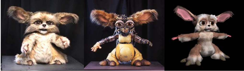
Figure 2: Leonardo, the robot and virtual simulator. Cosmetically finished (left), with mechanics exposed (center), and the animated model (right). Character design copyright Stan Winston Studio. Images copyright MIT Media Lab (left and right image) and Sam Ogden (center image).
