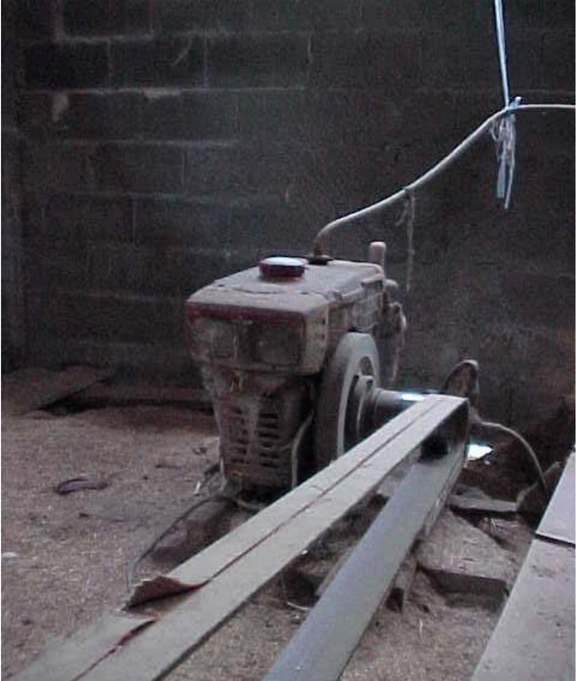
Figure 2--kubota motor driving rice mill
