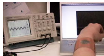
figure 2a: The bracelet is located at 14 inches away from the display – the oscilloscope shows the front-end output.
