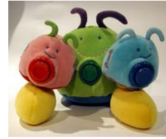
Figure 2: Three Program-a-Ball sensors (from left to right): LightBall , Programama and SoundBall .
