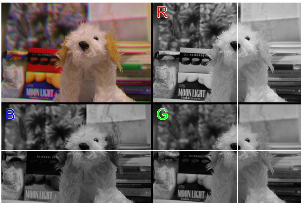
Figure 3.3: Example photograph taken with our lens, and its separated RGB planes. The white lines are superimposed to highlight the background color shifts. See Fig. 3.16(a) for a closeup view.
