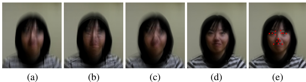
Figure 4.18: Motion-blurred face simulated from high speed camera images. (a) Static camera. (b) Coded exposure camera. (c) Motion-invariant camera. (d) Circular motion camera. (e) Facial feature point detection succeeded for the circular motion camera image (d) without deconvolution (and failed for the others (a-c)).
