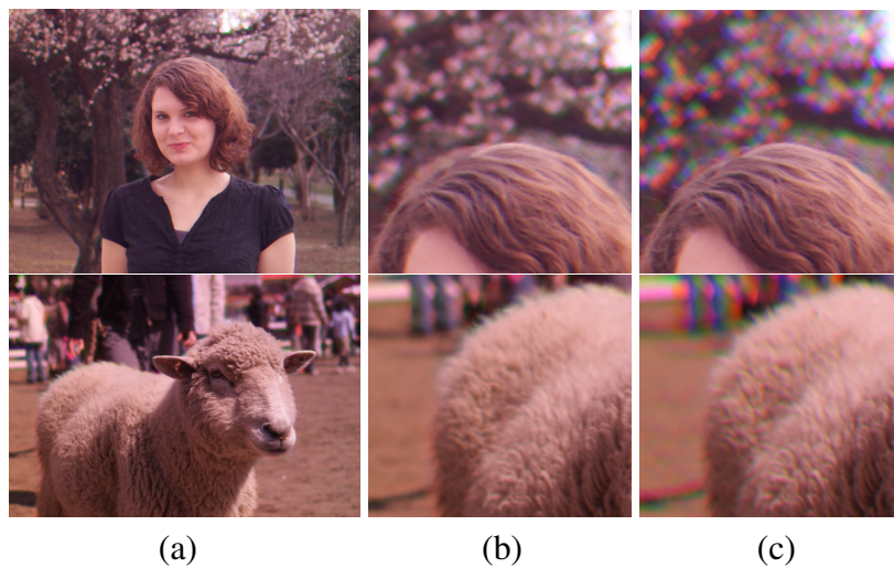
Figure 3.18: More color misalignment cancellation results. (a) Restored images. (b) Closeups of (a). (c) Closeups of the original.
