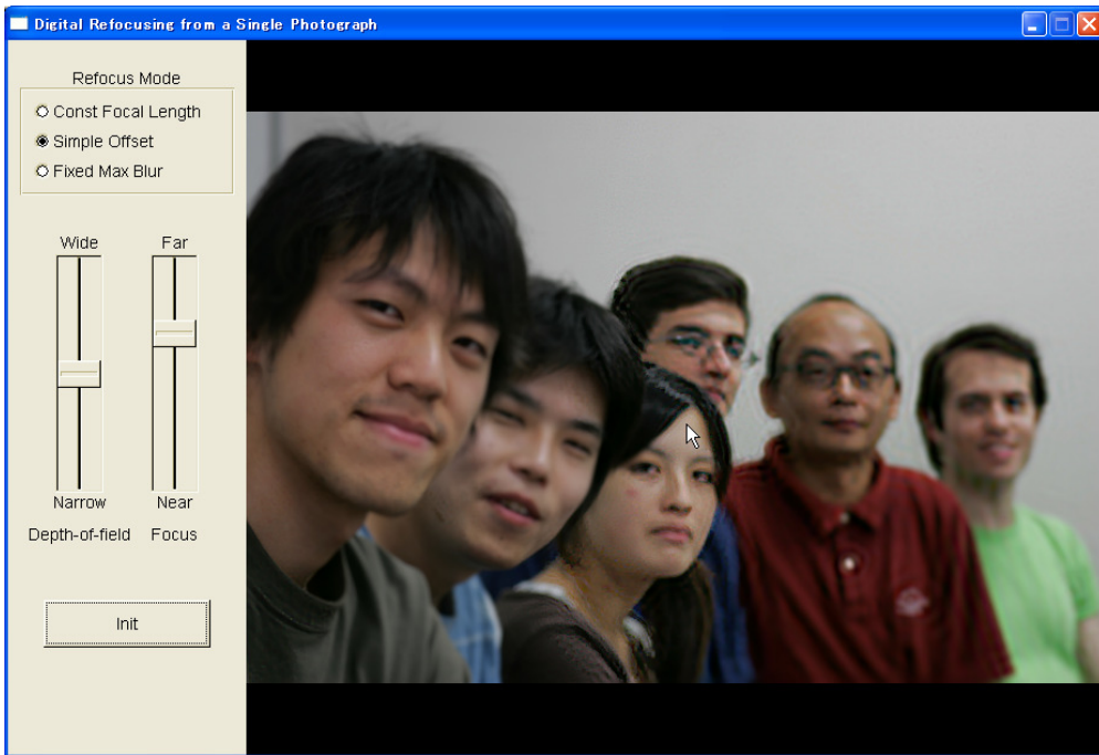
Figure 2.6: Screenshot of the interactive refocusing interface. The focused depth is immediately adjusted to the point specified by a mouse click.
