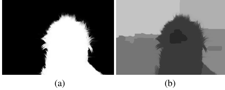
Figure 3.11: (a) Extracted matte for the toy dog image in Fig. 3.3. (b) Refined disparity map. Compare this with Fig. 3.10(a) top.
