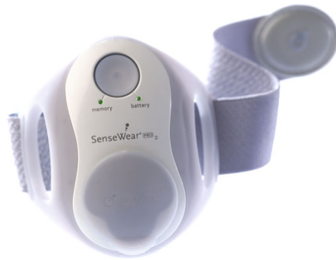
Figure 3-3: BodyMedia Sensewear Armband, measures 2-axis accelerometry, skin conductivity, heat flux and skin temperature
