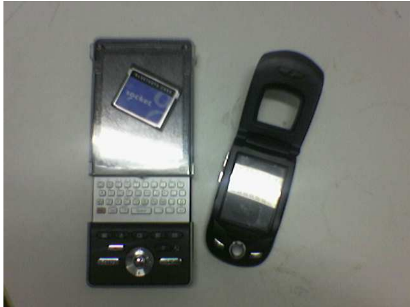
Figure 7-1: Bluetooth based Interest Networks system based on Zaurus SL 6000 or Motorola A760. The system is capable of real-time speech feature processing and bluetooth and wifi scanning.
