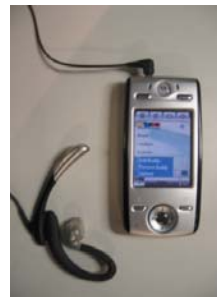
Figure 1. VibeFone application on an e680i mobile phone. The display fields from top to bottom are ‘mood’, ‘location’ and ‘buddies’
