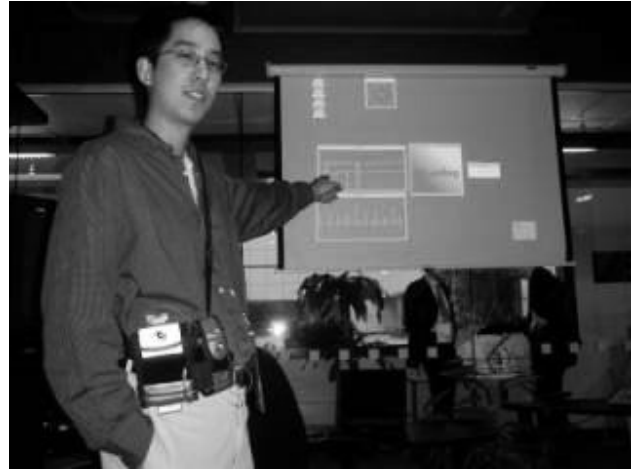
Figure 9: MIT.EDU application performing real-time FFT analysis and classification on accelerometer data, and wirelessly streaming real-time EKG/GSR/ temperature and classification results to a remote projector
