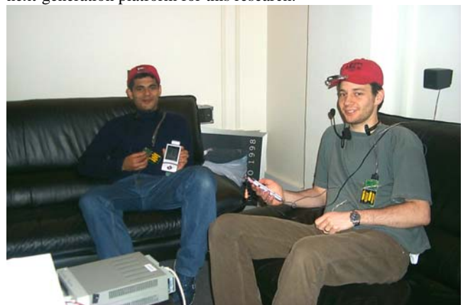
Figure 3. The GroupMedia system featuring a Zaurus PDA, Hoarder sensor board, bluetooth accelerometer [on hat], GSR leads and a microphone
