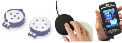
Fig. 2. Two Audio-haptic displays using embedded (a) MFTs made by Citizen (CMS-16A-07), used in a (b) vibrotactile “puff”, and (c) the Motorola A1000
