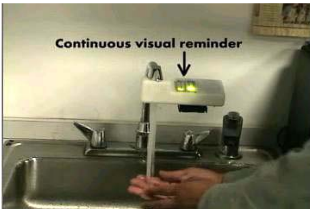
Figure 4. WaterBot offers continuous water usage feedback. It does not interfere with tasks performed at a typical sink.
