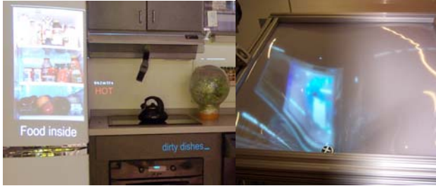
Figure 3. Information Annotation of the Kitchen (left) and video projection onto the surface of the SmartSink (right).
