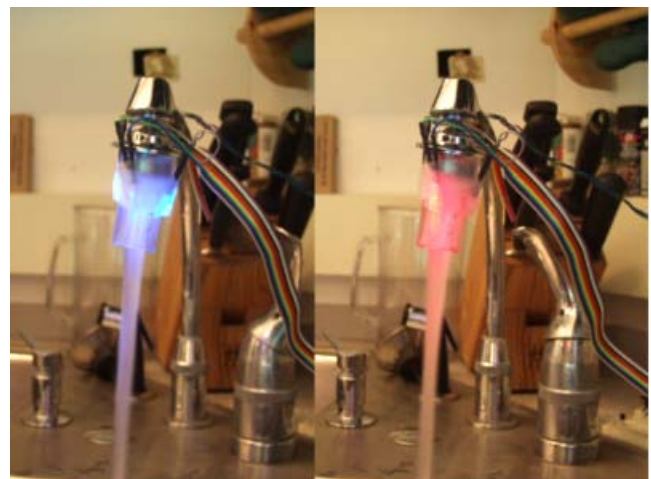
Figure 2. HeatSink cold (left) and hot (right).
