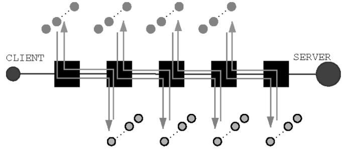
Fig. 6. Simulation in ns-2 with pareto cross traffic; 14 connections per link per direction.
