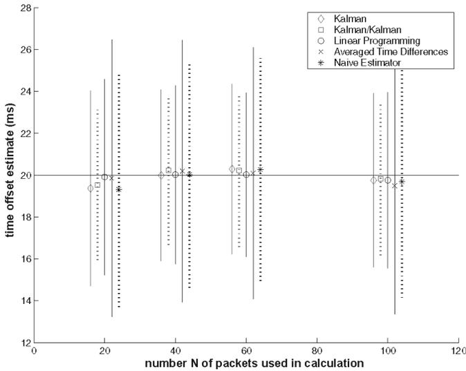
Fig. 5. Time offset estimate and standard deviation as a function of  $N$  (number of packets used), for Gaussian case.
