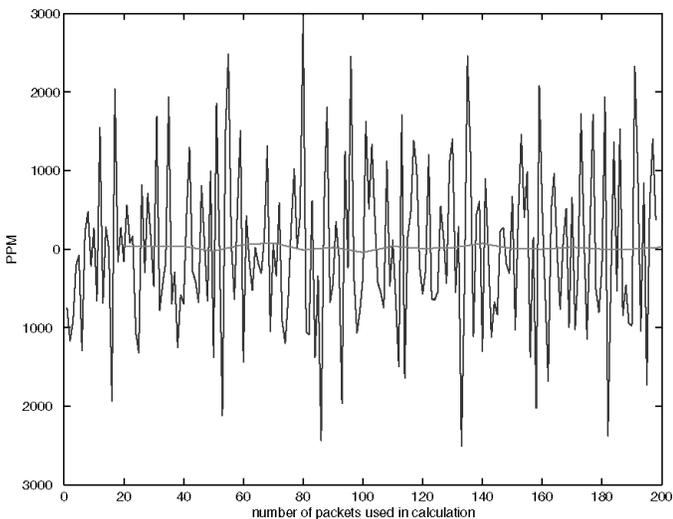
Fig. 10. Estimation of frequency offset  $\phi - 1$  using the ATD technique. Low pass filtering of data is also plotted.
