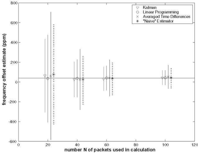
Fig. 4. Frequency offset estimate and standard deviation as a function of  $N$  (number of packets used), for Gaussian case.
