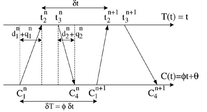
Fig. 2. Exchanging timestamps between client and time server. Notice that a time difference of  $\delta t$  according to server clock is translated to  $\phi\delta t$  according to client clock.
