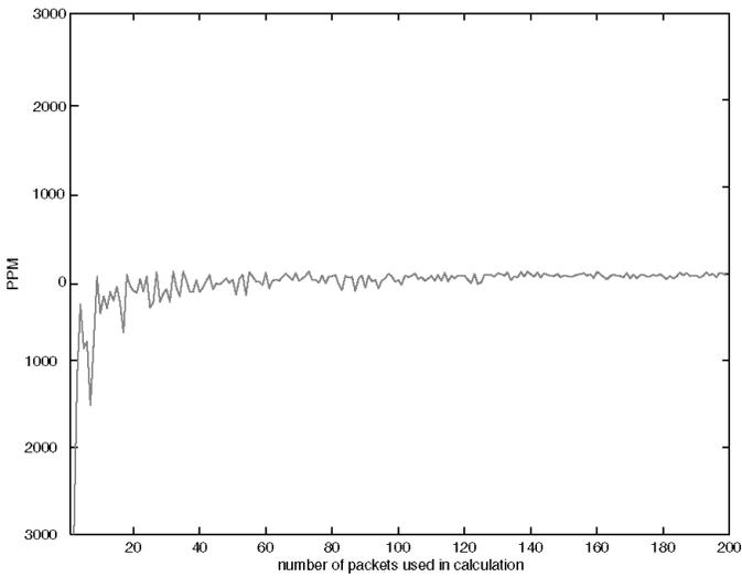
Fig. 9. Estimation of frequency offset  $\phi - 1$  using the Kalman filter for self-similar cross traffic.
