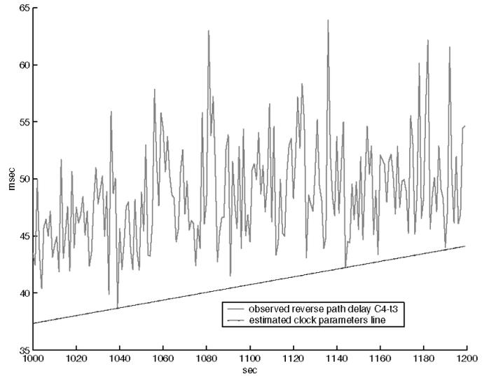
Fig. 11. Delay  $C_4^n - t_3^n$  from the reverse path and clock line estimation using LP for self-similar cross traffic.
