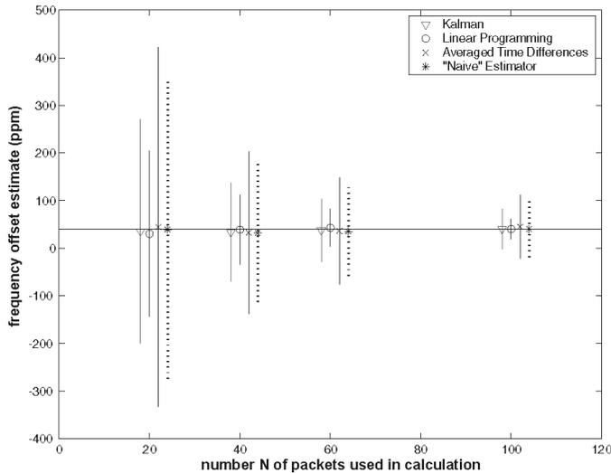
Fig. 13. Frequency offset estimate and standard deviation for self-similar cross traffic as a function of number  $N$  of packets used in calculation.
