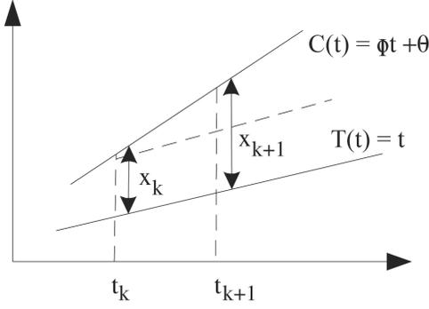
Fig. 1. Frequency offset  $\phi - 1$  and time offset  $\theta$  of  $C(t)$ , compared with the source of true time  $T(t)$ .
