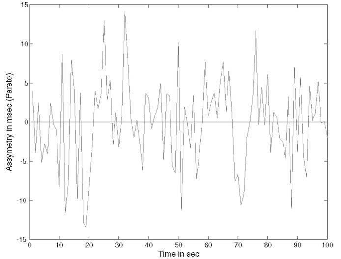
Fig. 7. Asymmetry between forward and reverse path with self-similar traffic.
