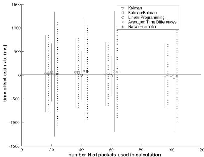
Fig. 14. Time offset estimate and standard deviation as a function of  $N$  (number of packets used), for self-similar traffic.
