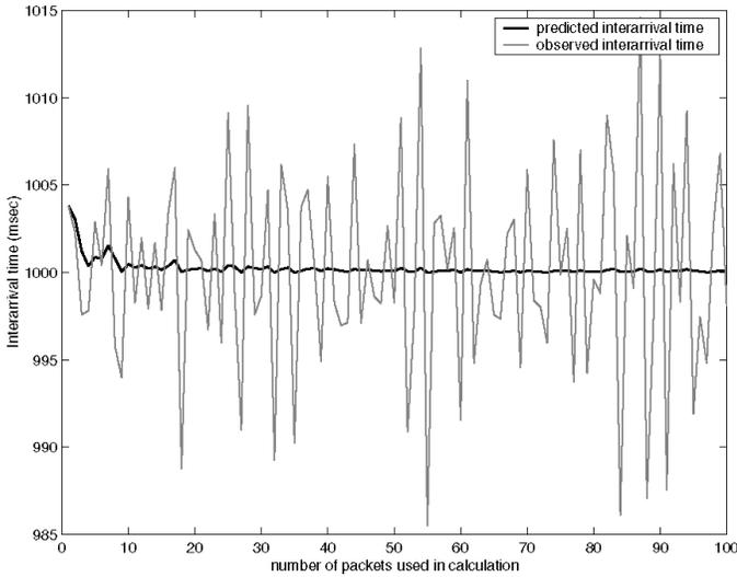
Fig. 8. Predicted interarrival and measured interarrival interval using the Kalman filter for self-similar cross traffic.
