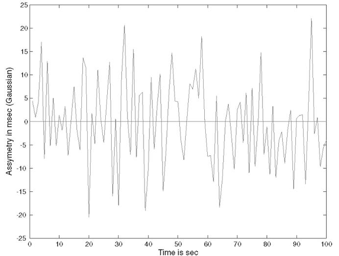
Fig. 3. Asymmetry of delays between forward (to server) and reverse (to client) path for Gaussian case.
