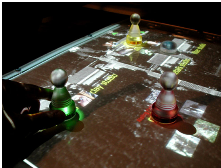
Figure 8: Created for the Digital Dialogues symposium held in September 2002, the first version of Tangible Spatial Narratives allows audience members to browse a database of documentary footage by manipulating small pawns on the surface of an interactive map. (Photo Credit: Ali Mazalek)
