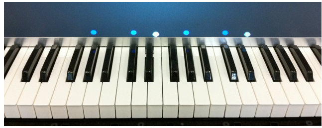
Figure 5: Dots indicating what keys are pressed at the corresponding keyboard
