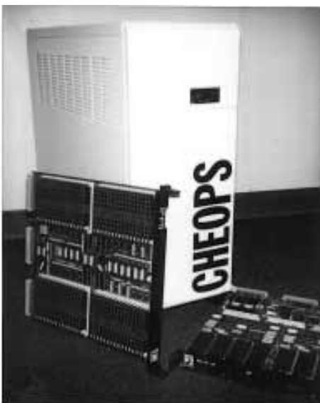
Figure 6: Nine-slot Cheops system in a floor-standing cabinet, with memory (left) and processor (right) modules removed. Smaller systems occupy horizontal card cages and can be placed underneath a video monitor.
