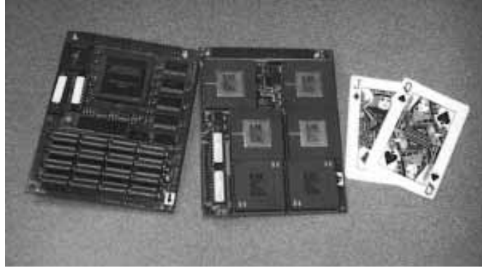
Figure 7: Stream-processor submodules, each containing two units (from left): remap/composite and DCT, dual multiply-accumulate/filter, playing cards for size comparison.
