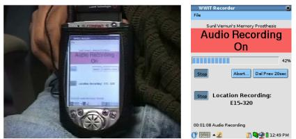
Figure 1: iRemember capture software running on iPaq PDA (top). Closeup of screen on the bottom
