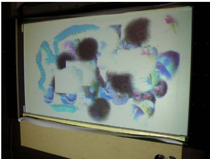
Back view of the touch panel overlay and projection. Note that the projection aligns on the top right corner (view from behind) with the overlay touch panel. The top right corner is also where the preview window is visible.
