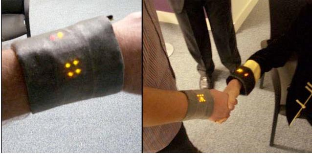
**Figure 1. The iBand and shaking hands with it.**
