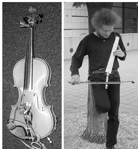
Figure 1: Left : Acoustic violin with mounted sensors. Right : Marching Cello
