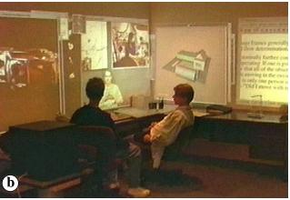
Figure 2: Our current implementation of the *office of the future*. (a) The cameras and digital light projectors are mounted near the ceiling using Unistrut material. (b) The walls consist of white foam-core board mounted on vertical posts. As shown in (b), they are used as display surfaces for a spatially-immersive display (SID).
