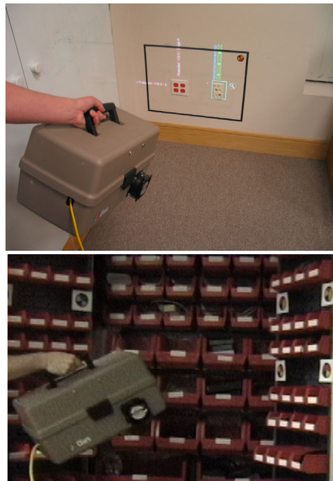
Figure 4: Context-aware displays. Top: augmentation of an identified surface; Bottom: guidance to a user-requested object in storage bins.
