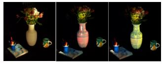
Figure 4: (Left) The underlying physical object is a white diffuse vase. (Middle and right) View-dependent effects, such as specular highlights, can be generated by tracking the user's location and projecting images on the vase.
