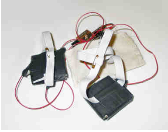
Figure 59: Shoe sensor assembly Two pressure sensors are attached to the sole of each shoe with elastic straps.
