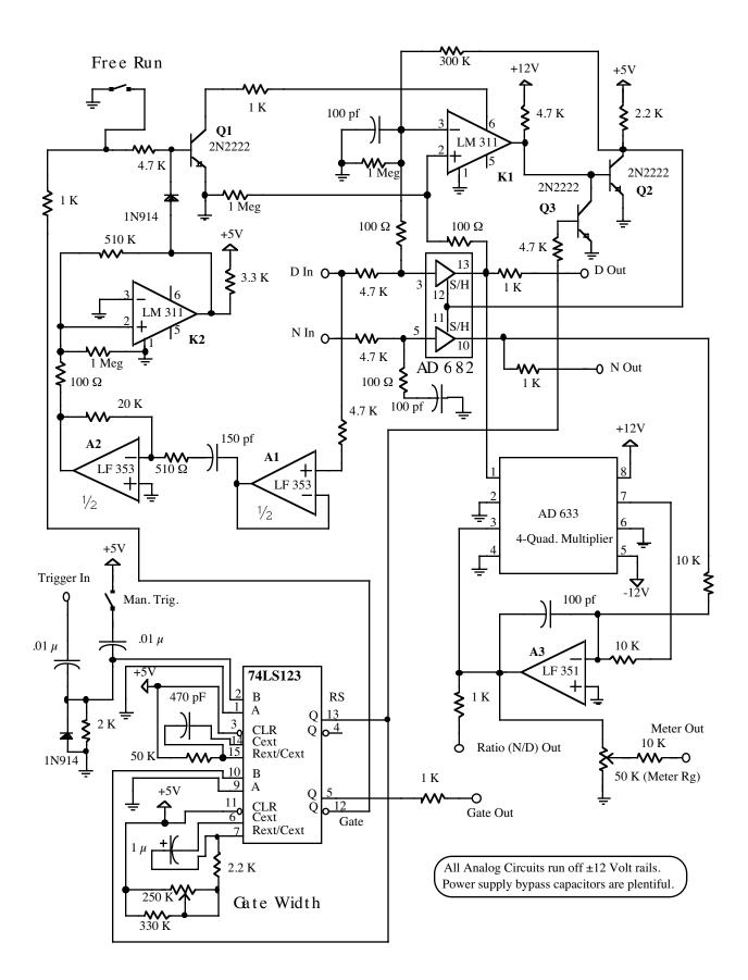
Figure 2: Gated Peak Denominator Ratio Generator (Bearing Estimator)
