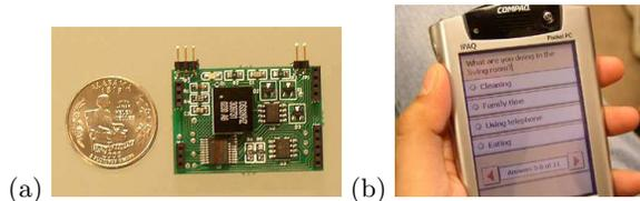
**Fig. 1.** (a) The state-change sensors that can be installed ubiquitously throughout an environment. Each device consists of a data collection board (shown) and a small sensor. (b) One screenshot from the ESM tool used in this work to collect training data on activities in the home setting.
