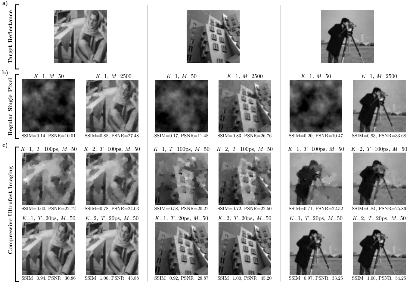
Fig. 11. Imaging with compressive ultrafast sensing for different targets. a) The target image. b) Result with regular single pixel camera with M = 50 and M = 2500 . c) Results with compressive ultrafast sensing with M = 50 for four design points with time resolution of T = 100 ps and T = 20 ps, and K = 1 and K = 2 . All reconstructions are evaluated with SSIM and PSNR. The results demonstrate the strong dependency on time resolution. Result for K = 2 and T = 20 ps shows perfect reconstruction on all targets based on SSIM. All measurements were added with white Gaussian noise such that the measurement SNR is 60 dB.
