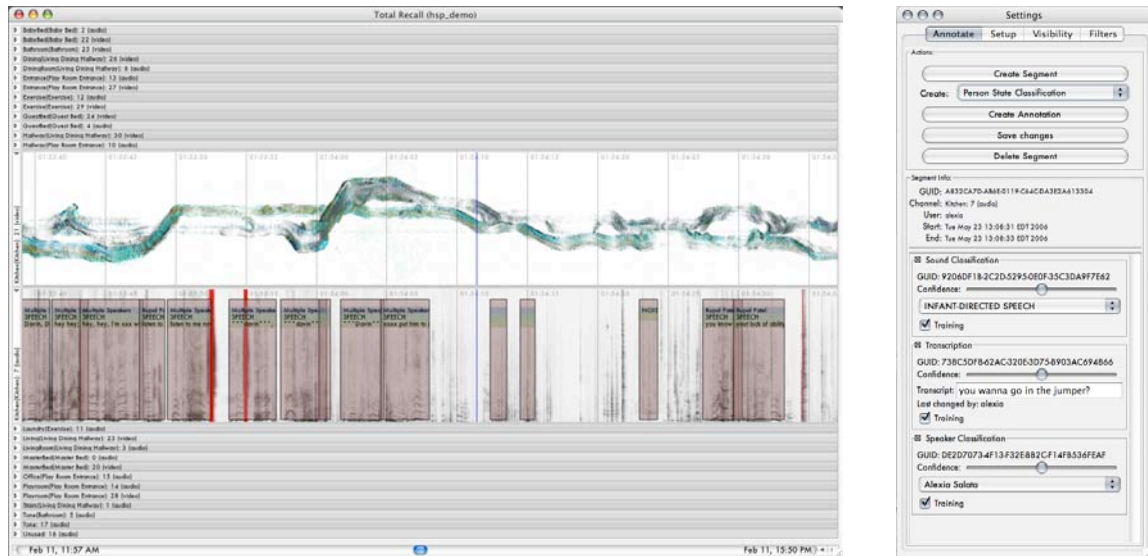
Figure 2: Screenshots of the TotalRecall system. In the left image, one video and one audio channel are being displayed. The video channel displays video volumes tracing two people moving in the kitchen. Below it, the accompanying audio track shows transcription and speaker ID annotations over spectrograms of the sound. The details window on the right shows additional information about the currently selected segment and its attached annotations.
